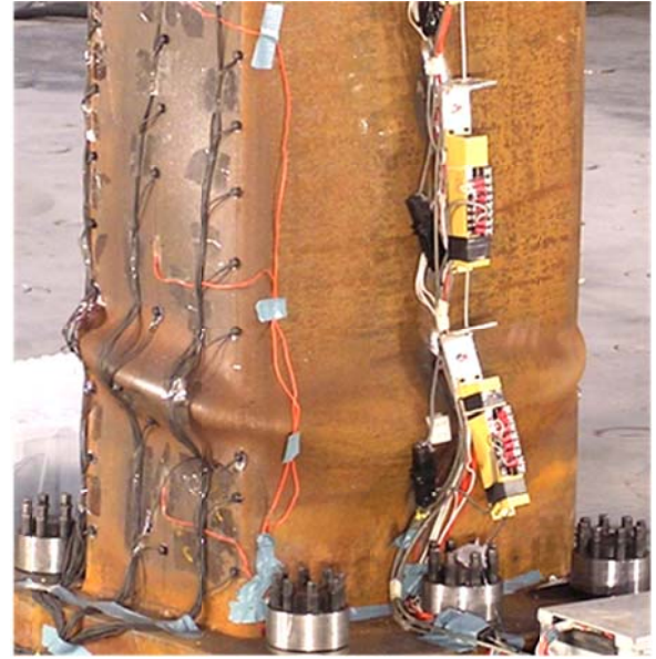
(b) Local Buckling Observed during Testing
